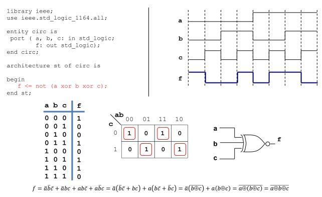
c) Complete the timing diagram of the following circuit: (5 pts)
