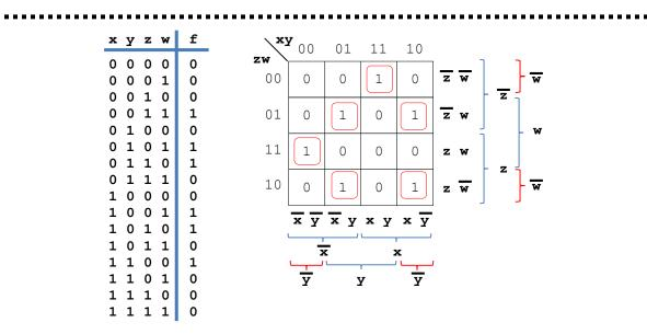
$f = \bar{x}\bar{y}zw + \bar{x}y\bar{z}w + \bar{x}yz\bar{w} + xy\bar{z}\bar{w} + x\bar{y}\bar{z}w + x\bar{y}z\bar{w} = \bar{x}w(y\oplus z) + y\bar{w}(x\oplus z) + x\bar{y}(z\oplus w)$
