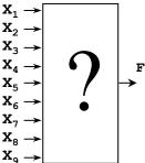
f = 1 when there are three 1's in a line. Note that there can be more than three 1's before we find three 1's in a line. So, we make f = 1 when a winning pattern is present regardless of the values of the remaining variables:
