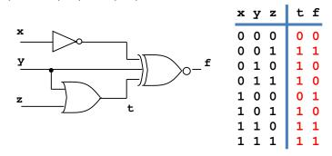
$f = \overline{\overline{x} \oplus y \oplus (y+z)} = \overline{\overline{x} \oplus (\overline{y}z)} = \overline{x}\overline{y}z + x\overline{\overline{y}z} = \overline{x}\overline{y}z + xy + x\overline{z}$
